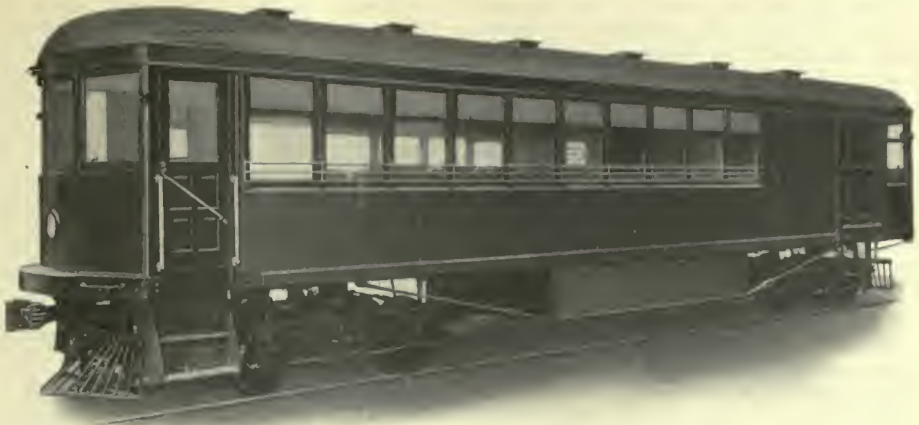
FIG. 443. STORAGE BATTERY CAR BUILT BY THE RAILWAY STORAGE BATTERY CAR COMPANY
